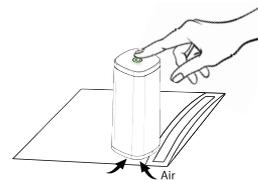
Gently touch the panel. Indicator light turns green. Pump starts working till air tight then automatically stops.
