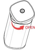
Open the battery cover by rotating it counter-clockwise.
